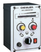
Chuck controller (with variable holding power and auto demagnetizer) B23-0106 (618M, 2A618, 612SP, 618SP, 818SP) Input: 110 V AC Output: 0~90 V DC
