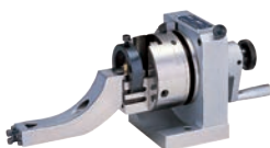
Punch former B07-0101 Diameter of the punch: 4~25 mm (0.16"~1.0") Length of the punch: over 22 mm (0.9")
