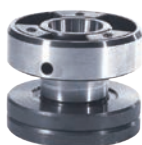
Wheel flange B05-0101 (618M, 2A618, 612SP, 618SP, 818SP, 2A / 3A818) Suitable for Ø205 x 6.35~20 x Ø31.75 mm (Ø8" x 0.25"~0.75" x Ø1.25") grinding wheel
